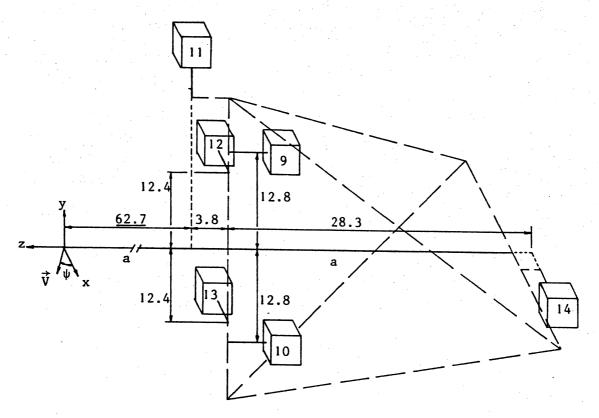
fig. 27.3. Schematic arrangement of the measuring elements 9 through 14. Broken lines: frame B, a: rotation axis,  $\vec{V}$ : direction of airflow, numbers with arrows: distances in cm.
