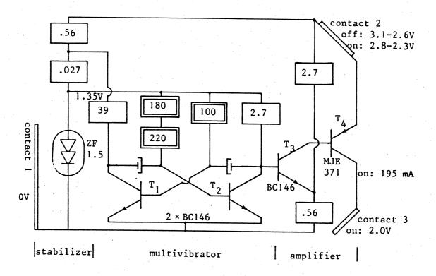
fig. 11.2. Circuit diagram. —[-= tantalum capacitor, luF roughly.  $\Box$  = carbon resistor,  $\Box$  = metal film resistor, numbers roughly indicate resistance in k $\Omega$ . T<sub>1,2,3,4</sub>: transistors.
