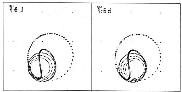
fig. 28.1. Bird's-eye view stereogram of boomerang flight ending 100 m below ground level.
