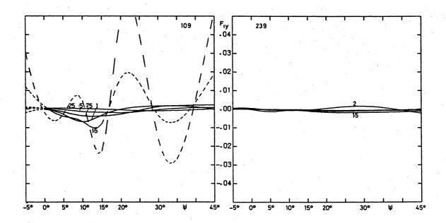
fig. 31.34. Boomerang WU, component  $F_{ly}$ . 109 = exp., 239 = theor.
