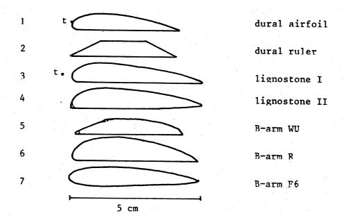
fig. 26.1. Cross sections of the wings used.
