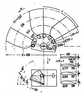
fig. 33.2. Taken from [Muesmann, 1958, p. 351]. Geometry of Muesmann's experimental axial-flow compressor rotor. Measurements in mm.
