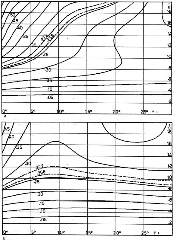
fig. 22.2 Contours of the function  $UT_{lx}/F_{lL}$  in the ( $\Psi$ ,U)-plane. a) for boomerangs 101. b) for boomerangs 195. Dashed lines indicate where the function equals  $\lambda$  for the plain resp.weighted version of the boomerang.
