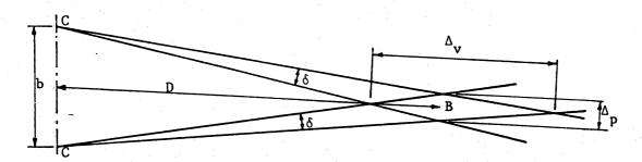
fig. 12.1. Uncertainty of boomerang's position in direction of viewing:  $\Delta_{\mathbf{v}}$ , and perpendicular to direction of viewing:  $\Delta_{\mathbf{p}}$ . C = camera, b = baseline, B = boomerang, D = distance boomerang from cameras,  $\delta$  = angular uncertainty in photographs.
