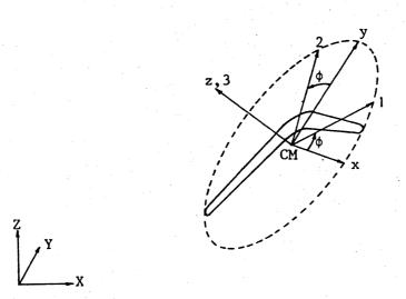
fig. 3.1. The three coordinate systems (X,Y,Z), (x,y,z), (1,2,3).
