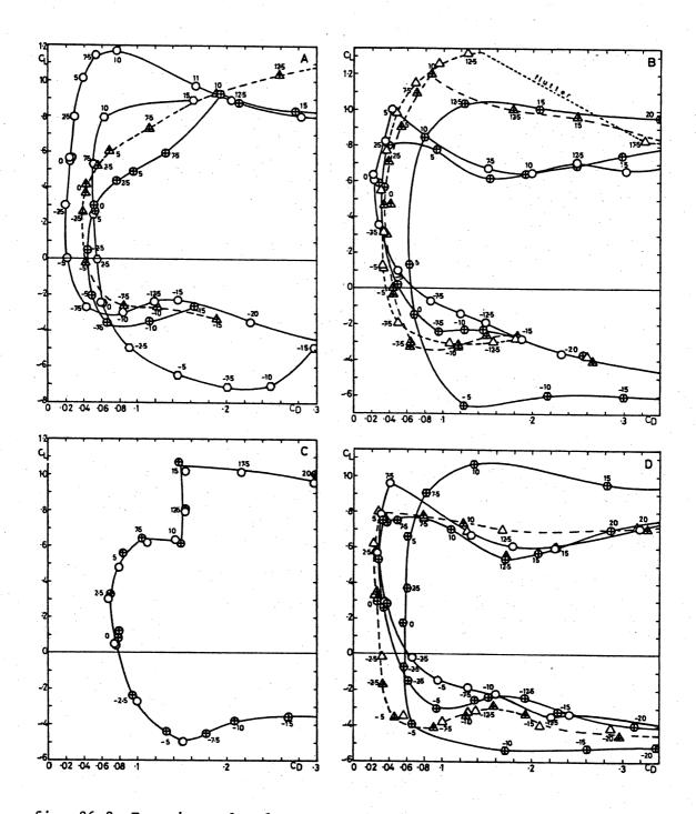
fig. 26.2. Experimental polar curves for 4 two-dimensional wings.
