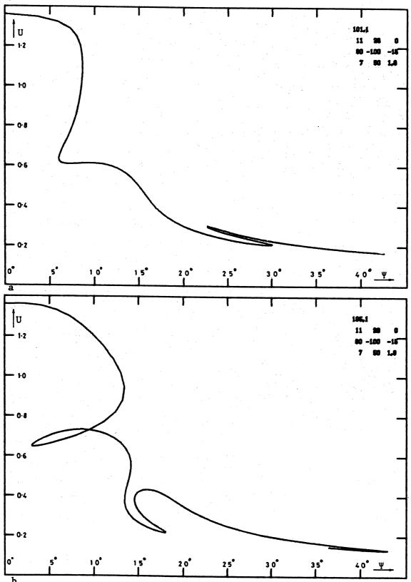
b fig. 22.1 (Y,U)-diagrams a) a flight by boomerang 101.1. b) corresponding flight by boomerang 195.1.
