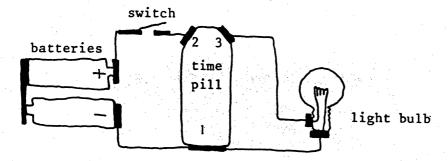
fig. 11.3. Connections between time pill, batteries and light bulb as mounted in boomerangs. == contact.
