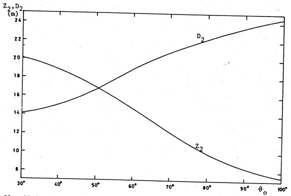
fig. 24.6. Maximum height  $(Z_2)$  and maximum horizontal distance before returning  $(D_2)$  vs.  $\theta_0$  for the flight paths of fig. 24.5.
