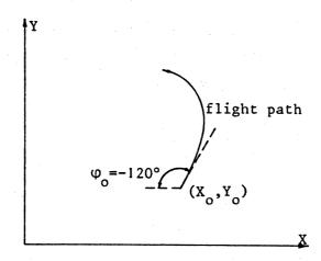
fig. 14.3. Example to explain the angle  $\phi_o$ . Bird's-eye view, boomerang launched at  $(X_o, Y_o)$  with  $\Psi_o = 0^\circ$ ,  $\vartheta_o = 90^\circ$ ,  $\phi_o = -120^\circ$ .
