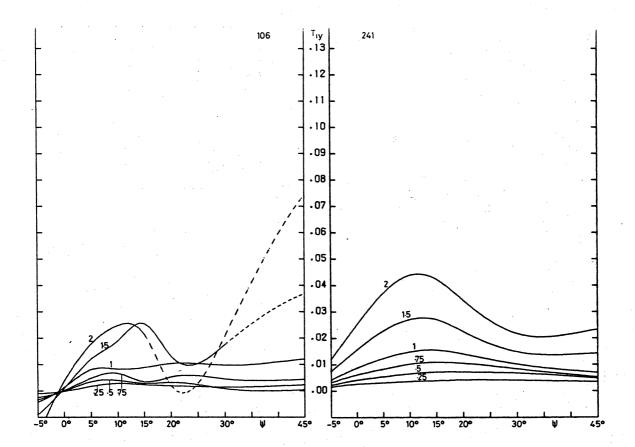
fig. 31.23. Boomerang L6, component  $T_{1y}$ . 106 = exp., 241 = theor.
