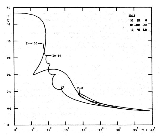
fig. 28.3.  $(\Psi, U)$ -diagram for the flight ending at Z = -100 m.
