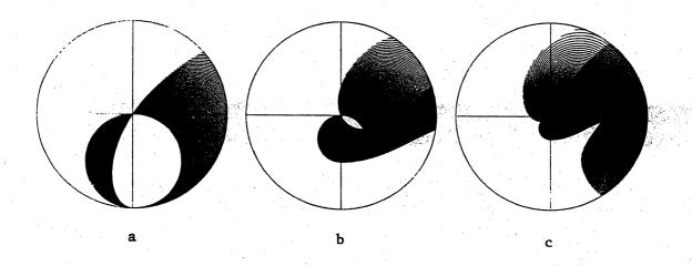
fig. 33.1. A rotating "straight stick" boomerang meets free vorticity shed by it previously in the shaded parts of circular region S. Rotation counterclockwise. Undisturbed flow from left to right.  $\psi = 0^{\circ}$ . a: U = 1, b: U = 0.5, c: U = 0.25.
