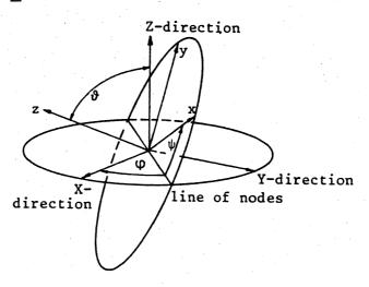
fig. 4.1. The Euler angles defining the relation between the (x,y,z)-and the (X,Y,Z)-directions.
