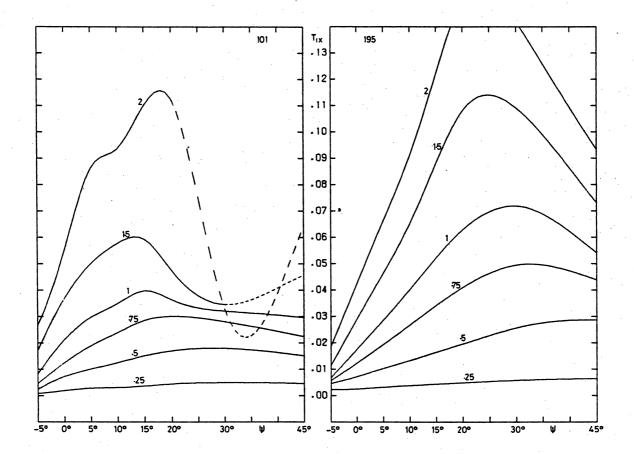
fig. 31.9. Boomerang L1, component  $T_{1x}$ . 101 = exp., 195 = theor.
