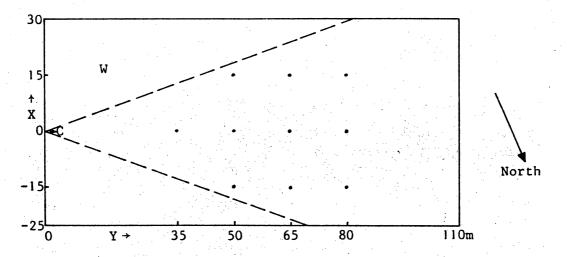
fig. 12.3. Field geometry. C = cameras, ---- = limits of field of vision, W = wind meters, . = field light.
