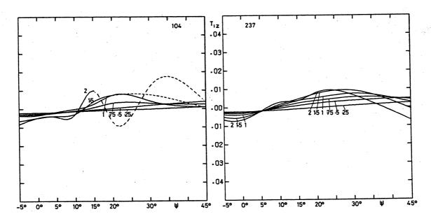
fig. 31.14. Boomerang L4, component  $T_{1z}$ . 104 = exp., 237 = theor.
