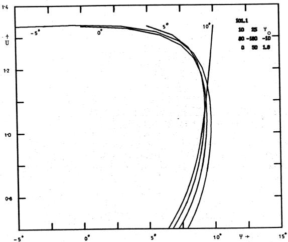
Fig. 27.3. Superimposed  $(\Psi,U)$ -diagrams for the first parts of the four flights discussed in this section. Boomerang 101.1 is launched at resp.  $\Psi_0$  = -5°, 0°, 5°, 10° and U = 1.34.
