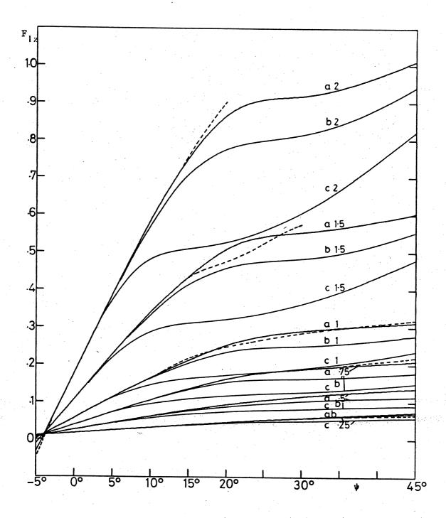
fig. 32.1. Component  $F_{1z}$  vs.  $\psi$ . Drawn curves: theory. Curves a: boomerang nr. 195,  $C_{L2}$  = 2.0. Curves b: boomerang nr. 217,  $C_{L2}$  = 1.6. Curves c: boomerang nr. 222,  $C_{L2}$  = 1.2. Dashed curves: experimental boomerang L1 (nr. 101) as far as different from nr. 195. Numbers with the curves denote U-values.
