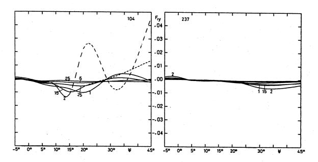
fig. 31.16. Boomerang L4, component  $F_{ly}$ . 104 = exp., 237 = theor.
