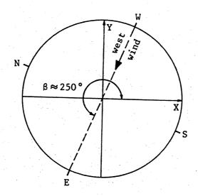
fig. 13.3. Wind direction with respect to (X,Y,Z)-coordinate system (after reflection). E.g.: for west wind,  $\beta \approx 250^{\circ}$  according to (8.8).
