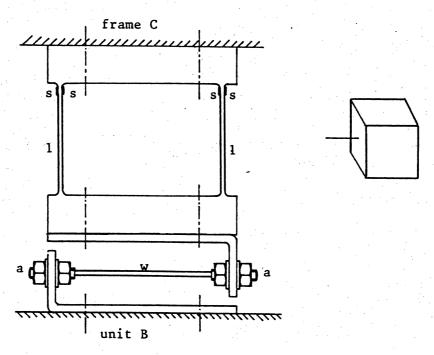
fig. 27.2. Measuring element. 1 = steel leafsprings, s = strain gauges, w = phosphorbronze wire, a = adjusting screws soldered to the wire. At right: symbolic representation of this element.
