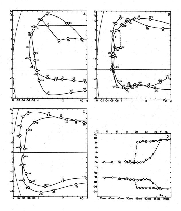
D. dural airfoil,  $\mathbf{C}_{L}$  and  $\mathbf{C}_{D}$  vs. Re at constant angle of incidence 5°.
