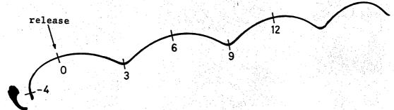
fig. 14.2. Instant of release of the boomerang in flight path photographs. Numbers denote time in units of 1/64 sec. from instant of release.
