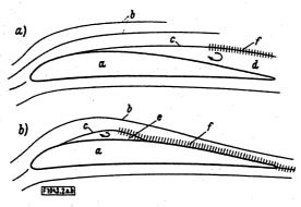
Fig. 26.4. Schematic picture of flow around airfoil (copied from [Kraemer, 1961a]). a) subcritical flow, b) supercritical flow. a = profile, b = streamlines, c = border stream line, d = dead water region, e = locally bounded dead water region ("Ablöseblase"), f = turbulent boundary layer.
