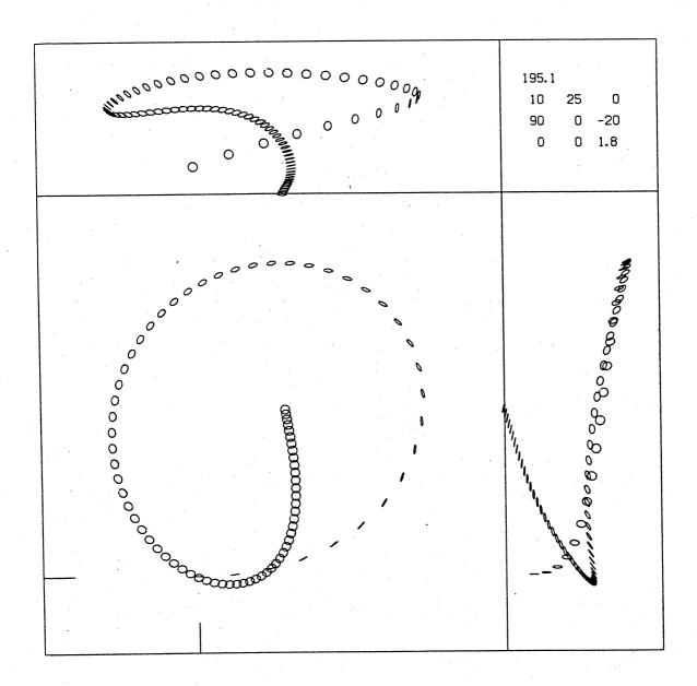
fig. 9.1. Example of a computed flight path. Three orthogonal projections are plotted. The boomerang's position is shown at intervals of 0.1 sec.
