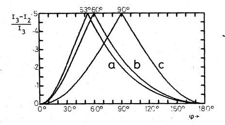
fig. 2.2. Graphs of  $(I_3 - I_2)/I_3$  vs.  $\phi$  for the cases a, b, c of fig. 2.1.
