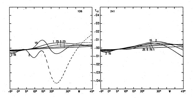
fig. 31.20. Boomerang L6, component  $T_{1z}$ . 106 = exp., 241 = theor.
