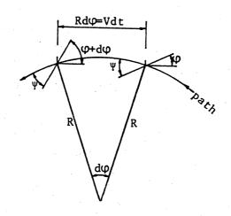
fig. 6.2.  $\frac{d\phi}{dt} = \frac{V}{R}$  for stationary  $\psi$ .
