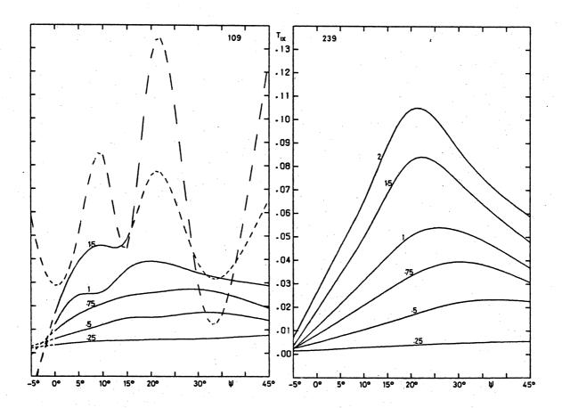
fig. 31.33. Boomerang WU, component  $T_{1x}$ . 109 = exp., 239 = theor.
