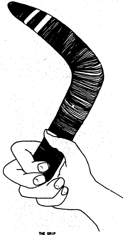
fig. 14.1. The grip for a right-handed thrower. (Copied from [Ruhe, 1972]). The boomerang may also be gripped at its other end, so that the free end point backwards.
